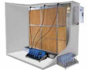
This newly developed in-duct humidification system can deliver up to 1,000kg/hr of moisture and 630kW of evaporative cooling to an air stream while operating on less than 0.3kW of electricity.
