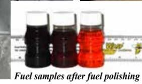
damage caused by water, leading to a complete generator failure; a high repair bill, and ultimately, no power. This is where fuel polishing comes in. It removes the contamination and maintains fuel in optimum condition.
