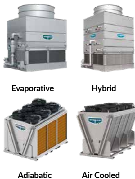
The four primary types of closed-loop heat-rejection equipment are evaporative closed-circuit coolers, hybrid closed-circuit coolers, adiabatic coolers and dry coolers. The cooling load of the system, available equipment space, sensitivity to water consumption, maintenance requirements, and project budget should determine which option is best.
